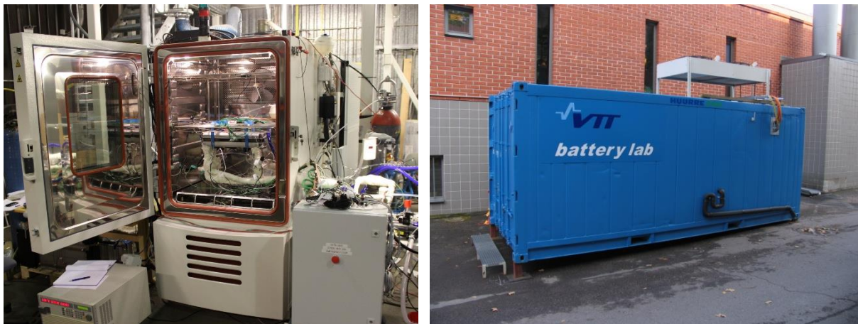
Figure 6: Left: 1 kW S2 stack during freeze testing in a climate chamber. Right: VTT climate chamber suited for testing larger systems.
